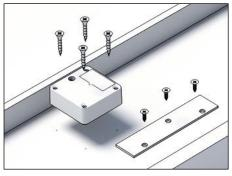
Remove all hardware and disassemble Shelf Top Assembly from Bottom Assembly for final finishing or painting of Shelf.
