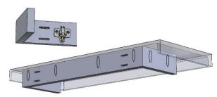
Locate circular Strut Mount Bracket and location on Cleat where bracket will be installed. Transfer holes for mounting bracket. Hole orientation is not critical. Glue and Pin Nail miter assembly together. Clamp and let dry.
